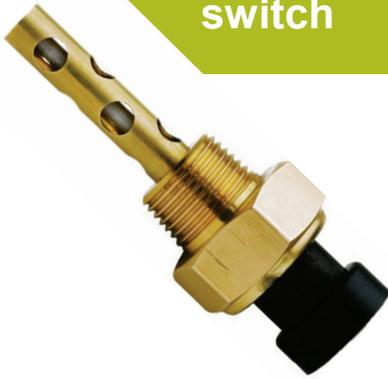
The **Model S86** is an active device which is designed to give an alarm signal if fluid falls below a preset level. It will only signal an alarm after a few seconds of low level to eliminate false alarms due to turbulence.
