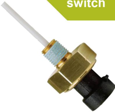
The **Model S98** is an active device which is designed to give an alarm signal if fluid falls below a preset level. It will only signal an alarm after a few seconds of low level to eliminate false alarms due to turbulence.
