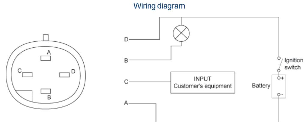
Note: Pin B has the option to be a communications port rather than an alarm if factory configured at the time of ordering.
