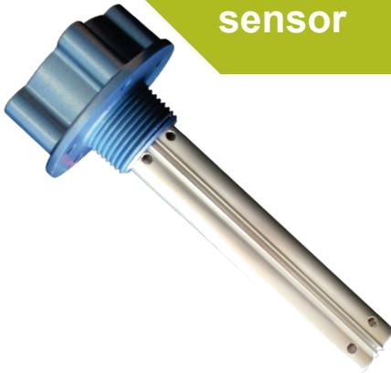
The **Model T/LL350** series is a range of highly advanced sensors for continuously measuring the contents of a tank. The unique feature of the T/LL350 is that it recalibrates itself when a liquid with a different dielectric constant is used. For example, if it is used in a tank of conventional diesel, then the user can refill with bio-diesel and the sensor will correct the output level automatically.
