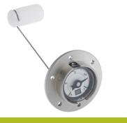
The **G/LL28 Series** is a simple, robust, mechanical liquid level contents gauge using a float to move the dial pointer via a magnetic coupling. This prevents ingress of the tank contents into the indicator capsule.
