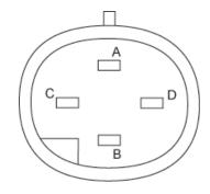
NOTE: Pin B on configuration 1, 2 and 3 is used for 4-20mA loop. On configuration 4, 5, and 6 the connection is used for Low Level Alarm.
